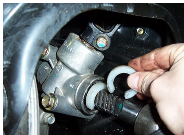
Install steering stops to the pinion shafts on each side.
